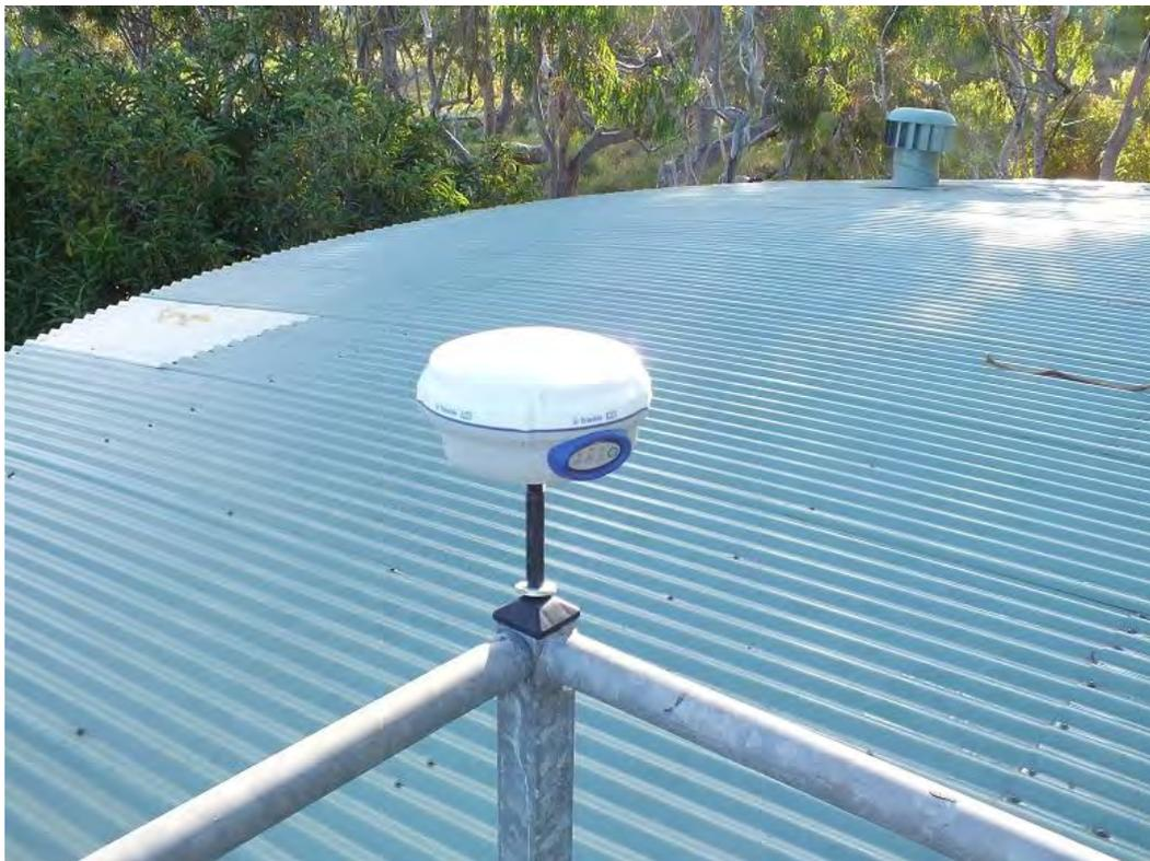
**Figura 2.1-4 Antena Base instalada**
