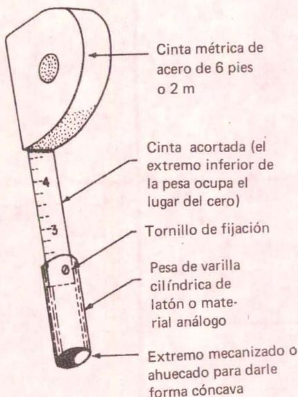
Fig. 3-5. CINTA METRICA CON PESA PARA MEDIR EL NIVEL FREATICO
