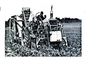
Mechanical snap bean pod harvester. Mechanical harvesting of vegetables for processing is a once-over, plant-destructive operation. Only the pods of acceptable size and quality at harvest are usable for processing. Uniformity among plants is necessary for high, reliable yields of quality produce.
