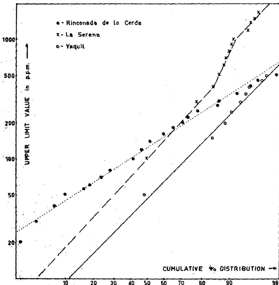
Fig. 4. Cumulative percentage distribution for copper from soil surveys from La Serena, Rinconada de lo Cerda and Yaquil.
