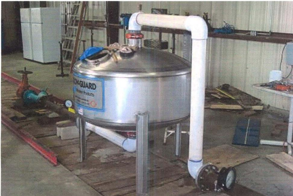
**Foto 14: Banco de prueba de filtros de grava, Center for Irrigation Technology, California State University – Fresno.**
